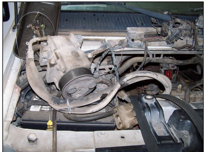
FIG 12 : A/C Compressor Moved Off Engine
