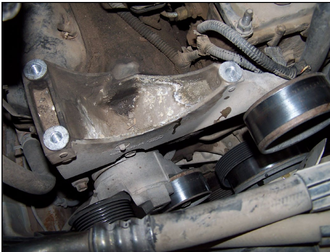
FIG 9 : Belt Tensioner – Lower Center of Photo
