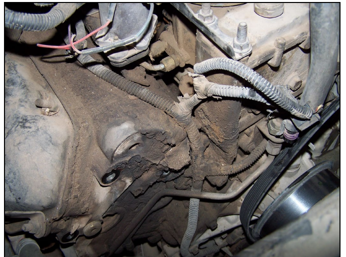
FIG 10 : Alternator Bracket Removed
