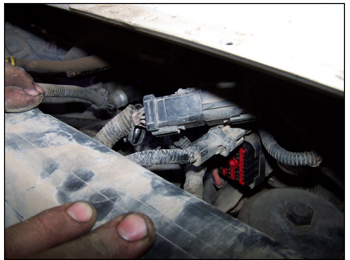
FIG 4 : Connectors Behind Cowl Wiring Harness
