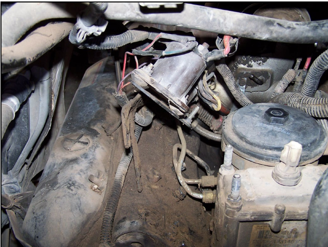
FIG 17 : GP Bracket Moved – Fuel Lines Exposed
