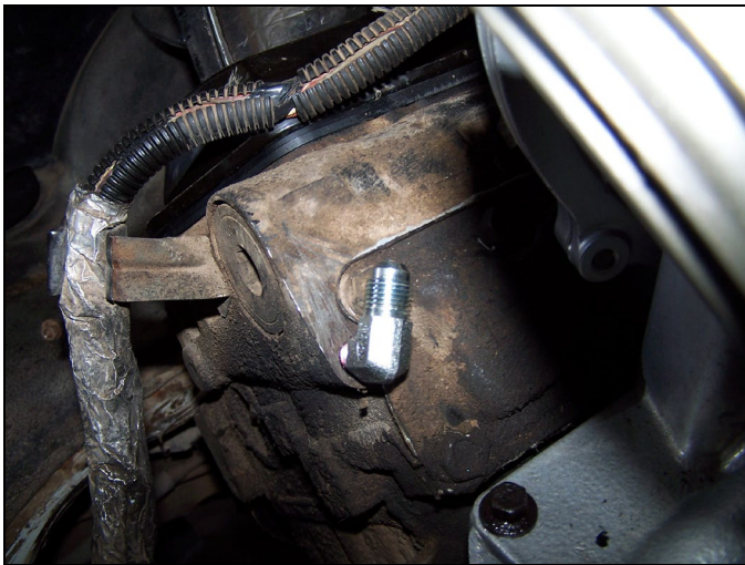
FIG 21 : Driver Side Rear Fitting Installed
