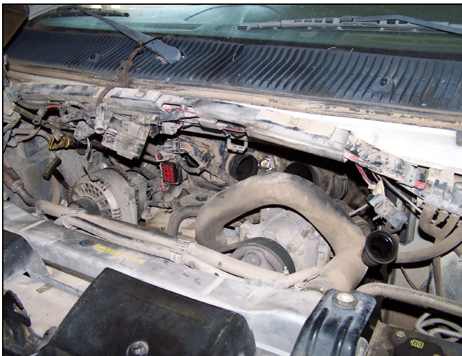
FIG 5 : Cowl Harness Pulled Up Out of Way
