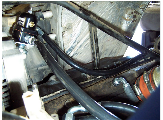
FIG 34 : Driver and Passenger Hoses Connected to Reg
