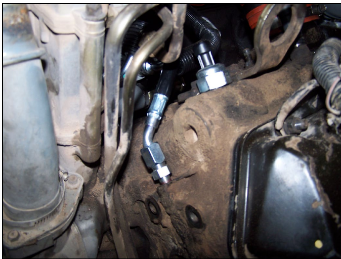
FIG 27 : Drivers Front Feed Line Connected
