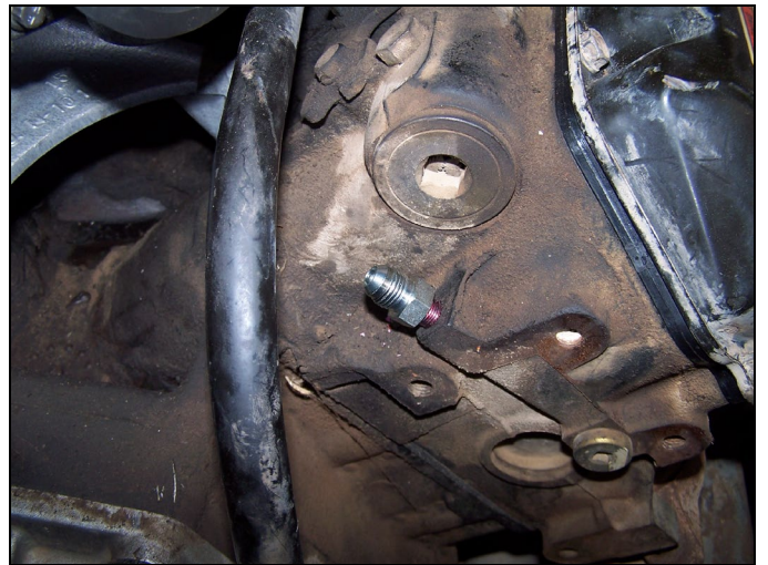
FIG 22 : Passenger Side Rear Fitting Installed
